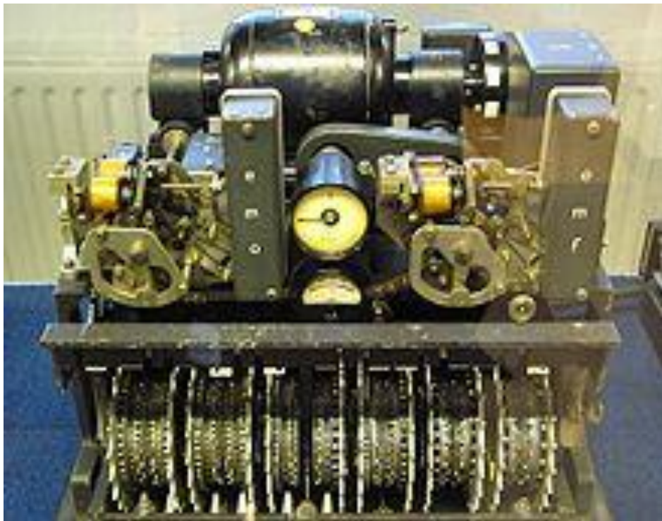
German Lorenz cipher machine, used in World War II to encrypt very-high-level general staff messages
